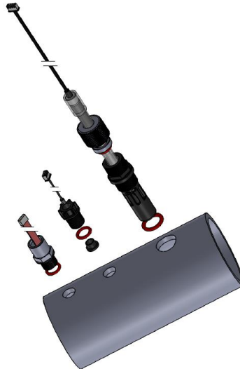
Figure 44 - Sensors on Threaded 3" Pipe
